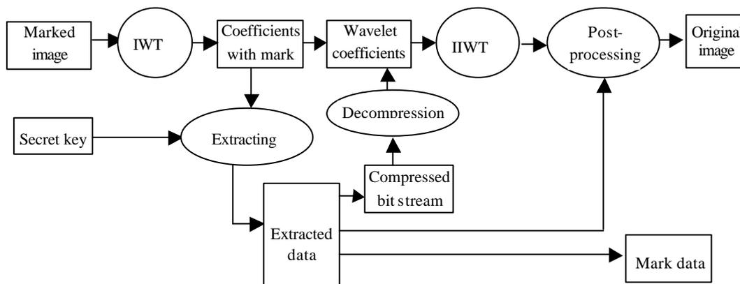
Figure 3 Data extracting algorithm (IWT denoting integer discrete wavelet transform, IITWT inverse IWT).
