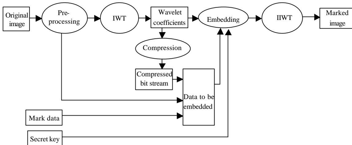
Figure 2 Data embedding algorithm (IWT denoting integer discrete wavelet transform, IITWT inverse IWT).
