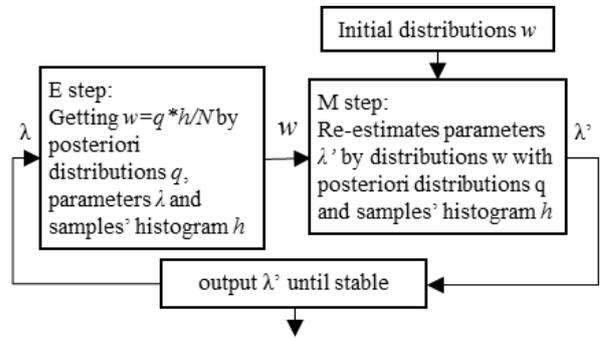
Figure 3. Block diagram of proposed novel EM
