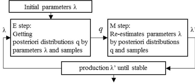
Figure 1. Block diagram of conventional EM
