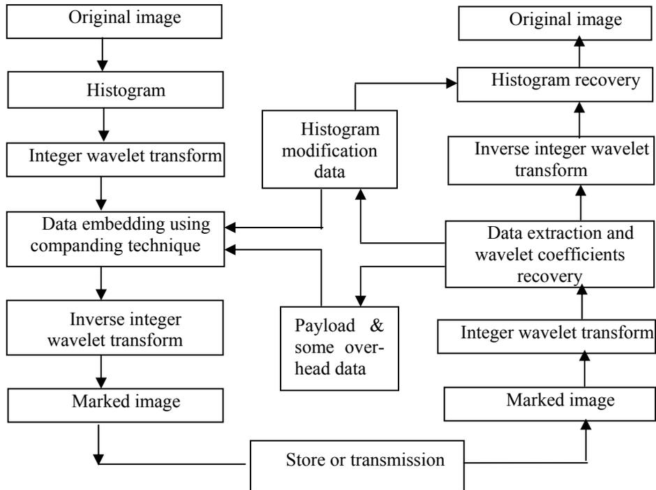
Figure 2. Block diagram of reversible data hiding diagram. Left: data embedding, Right: data extraction.
