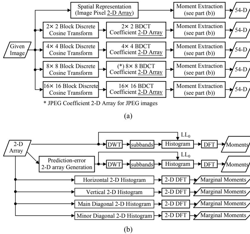
**Fig. 6.** Feature generation block diagram of Chen et al.'s method. (a).General block diagram; (b).Moment generation block diagram
